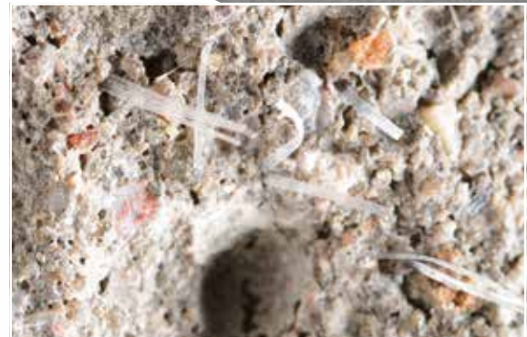
Enlarged view of FASERFIX® concrete. The photograph clearly shows the fibres which give the material its great strength.
