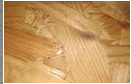
Woodchip board achieves its great strength with the help of a closely interlinked fibre network.
